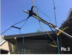
**Pic 3** is a close up of the assembly ready to be raised ... I put the wire spreaders in place to keep the wires safely apart.
