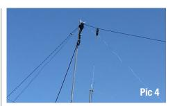
**Pic 4** is a zoom shot of the mast. I have yet to get those wires exactly where I want for inverted V best practices. The V is up about 25-30 feet high.
