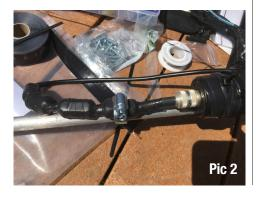
**Pic 2** is the feed line connection before I taped that up too. I have some beads on it just because and used that bead to throw a hose clamp on to attach it to the top of the mast. The coax reverse runs to the top of the mast and then back down ... again to keep the strain off, simply letting the coax get tugged on.
