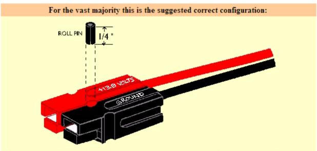
"Housings should be mated according to the diagram above, viewing from the contact side (opposite the wire side), tongue down, hood up, RED on the LEFT, BLACK on the RIGHT. Also notice the 3/32-inch-diameter roll pin, 1/4 inch long, is used to keep the housings from sliding apart."
